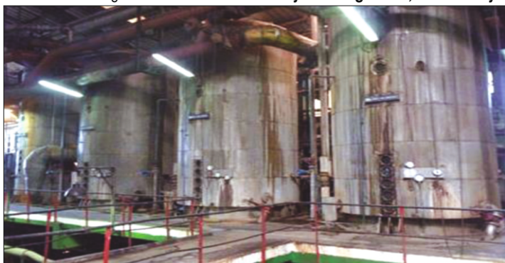
Sugar Cane Evaporating Process in Evaporators Gayathri Sugar Ltd., Kamareddy
